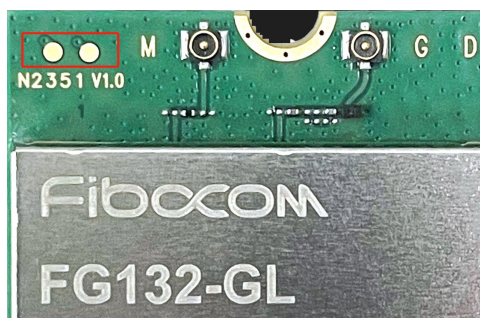
Figure 11. forced download test points
